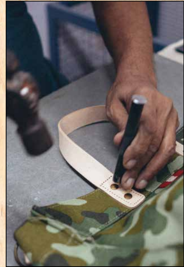
NIZAMUDIN APPLYING BRASS RIVETS BY HAND TO OUR MINI BOX TOTE
