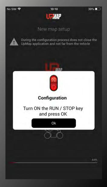
Turn the RUN / STOP button on the bike to RUN and press OK
