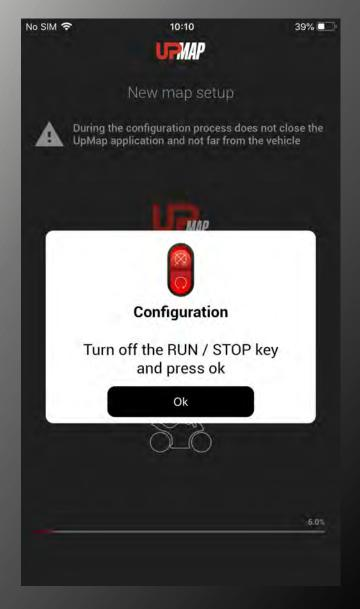
Turn the RUN / STOP button on the bike to STOP and press OK
