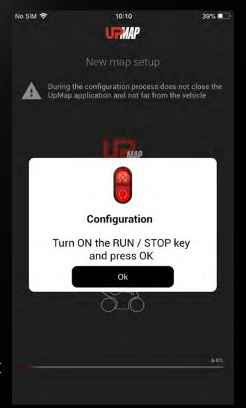
Turn the RUN / STOP button on the bike to RUN and press OK
