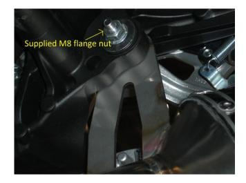
6. Check for clearance, tighten all mounting hardware, and re-attach your O2 sensor.
