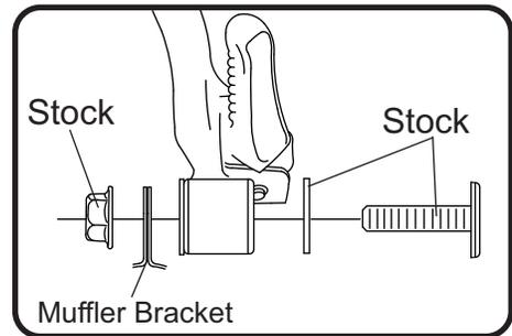
4. Torque muffler mount bolt to factory specification.
