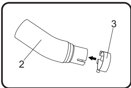
2. Install (No. 2) 11801-435, tailpipe over the stock header outlet.
