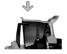
In ALUS mode, pull the gauge against the chosen correction plane on the inside of the rim, press ( to automatically input.
