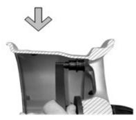
Do not return the gauge and keep pulling the gauge until it is against the chosen correction plane on the outside of the rim, waiting.....
