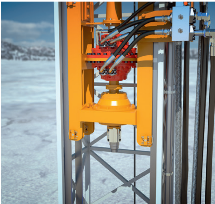
▲ Drilling /top drive
