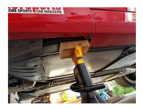
2. Put jack under oil pan and use a 2x8 (or something similar) to distribute the load. Do not lift the engine yet but raise jack so it makes contact with the oil pan and wood stays in place.
