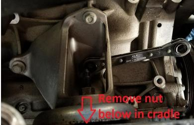
5. Raise engine using jack until you can get the bracket and mount assembly out as one. You may need to use a pry bar to compress the stock mount. Keep an eye on intake manifold clearance to cowl. Do not raise engine too high or contact will result. Front cradle may have to be lowered by loosening the four nuts to gain additional clearance.
