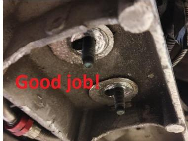
3. With nuts removed jack the transmission to a height where it barely touches the rear tub of the trunk area above. It's not necessary to jack the trans quite this high but every little bit of clearance helps to remove the old diff mount. And yes, you can do this even if you're using our Vulcan Motor Mounts with the single bolt-thru design.
