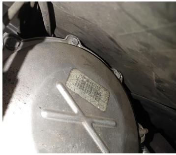
4. Remove the bolts holding the diff mount to the differential using a 15mm wrench or socket. You can lift the hard brake lines up and squeeze a socket underneath them to remove the bolt on the passenger side
