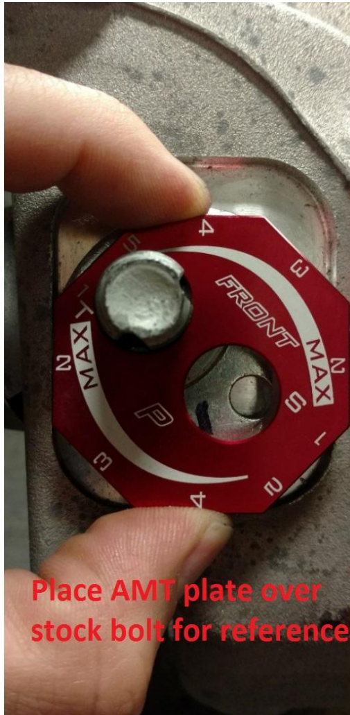
AMT plate is installed in Position T2
