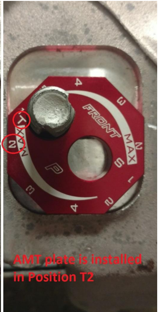
Place AMT plate over stock bolt for reference
