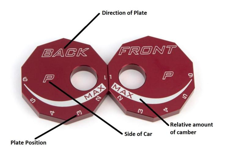
**Side Of Car** – Each pair of plates is marked with either a "P" or a "D". All plates with a "P" on them will be installed on the Passenger side of the car and plates with "D" on them will be installed on the Driver side of the car.
