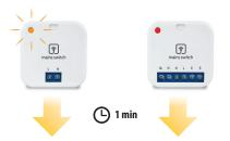
When the transmitter exits the pairing mode, it sends a signal to the receiver. LED diodes on both devices are green now. The devices are ready for work.
