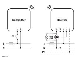
When S1 transmitter contact is closed, receiver sends 230V AC (SL output).
