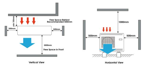
Intake and outlet should not be obstructed. The wall the unit is to be mounted on should be strong enough to bear the weight and vibrations of the unit.
