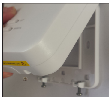
Align the front housing at the top edge.
