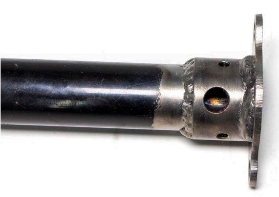
Connect the steel rear coupler to the back of the EPAS system using the provided bolts. Test fit the steering column and EPAS motor in place and clock the motor to your desired position.
