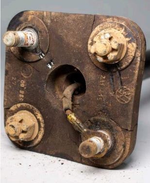
Before cutting, remove the wire running through the shaft. The eyelet securing it in place is located underneath the connector.
