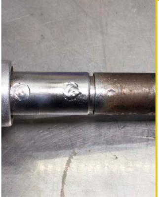
Insure the provided splined coupler is fully seated onto the lower section of the steering shaft and weld in place.
