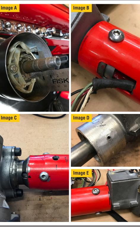
Reassemble the complete steering column/EPAS unit. Repeat steps for drilling and tapping the 3 set screw holes. Note the turn signal stalk should be at 9 o'clock, and the EPAS motor around 2 o'clock, so keep that orientation in mind when positioning the upper column. (*Image F*)
