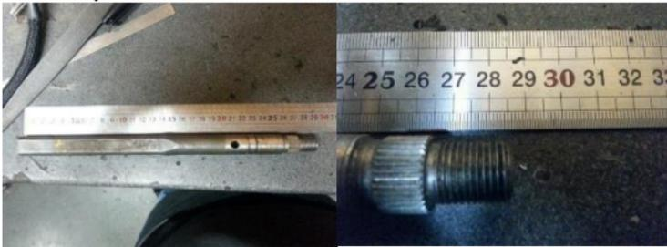
5. Attached the inner shaft into the  $\frac{3}{4}$ '' DD cupler on the end of the EPAS motor, that is welded onto the motor. Be sure to tighten down the 2 set screws on the cupler that is welded onto the motor, to hold the shaft in place.
