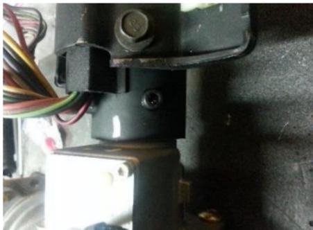
9. Once the motor is "clocked" and marked, return to the bench to drill holes in the column. With the drill bit provided from EPAS, drill 3 holes at 120 degrees each. (Photo above shows proper positioning of set screws. Arrows.) the Tap with the EPAS tap provided. Insert the 3 set screws, also provided by EPAS.
