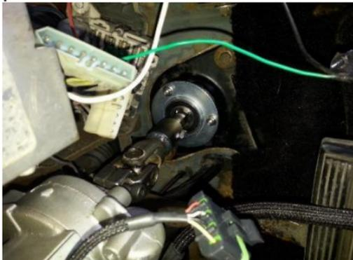
14. With the 1" DD shaft, slide into the  $\frac{3}{4}$ " DD, and the ujoint going to the steering box. Both  $\frac{3}{4}$ " DD shafts should sit inside of each other by about 2". Re adjust if needed.
