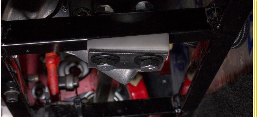
For motor installation, angle the motor and push the splined steering shaft through the upper column bearing. Sliding the 3/4" DD into the lower 1" DD. Optionally, remove and reinstall upper column bracket with bearing.
