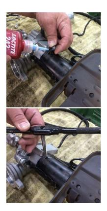
To begin reinstalling your column you will first need to clock and mark the column for staking. Place the column and motor assembly in the vehicle and set the motor at the desired position marking the tap locations.
