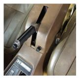
The wires will run inside the console, the power wire will go from front to back blue terminal and the torque sensor from back to front Delco pack and small red ignition wire from back to front as well.
