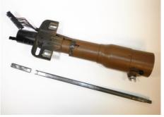
Then cut 3 ½ " of the steering shaft, the shaft will then slide into the ¾" DD on the electric motor and tighten the two set screws.
