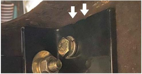
The side of the mounting hardware that has **TWO** notches goes to the **drivers** side.
