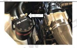
4:(9mm Inlet) Secure Oil catch can fitting with Teflon tape
