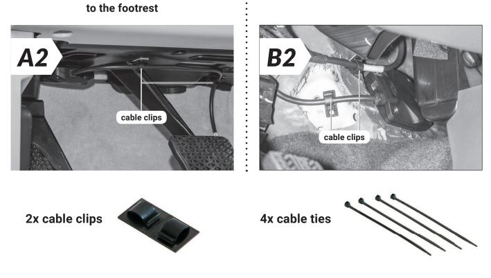
• Use the cable clips and/or cable ties to secure the cable between the Brainbox and the Controller, ensuring that nothing interferes with the pedals.
