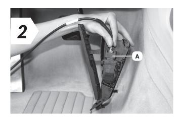
• Attach connector **A** from the Brainbox to the gas pedal sensor.
