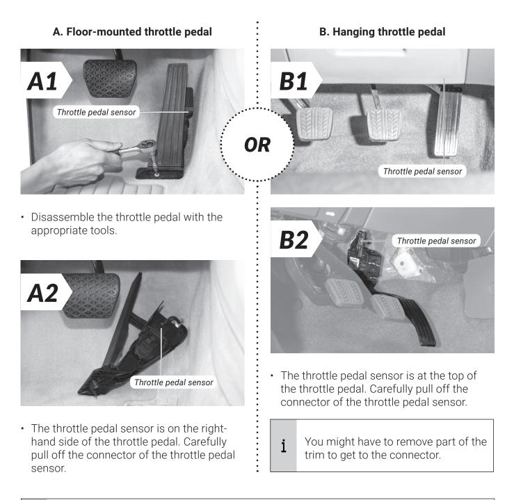
If you need assistance in detaching the throttle pedal sensor connector: see the additional instructions **"Detaching the connector correctly".**
