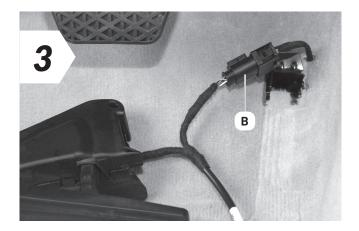
• Now attach connector **B** to the connector you pulled off the gas pedal.
