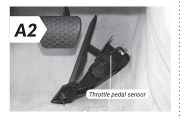
The throttle pedal sensor is on the righthand side of the throttle pedal. Carefully pull off the connector of the throttle pedal sensor.
