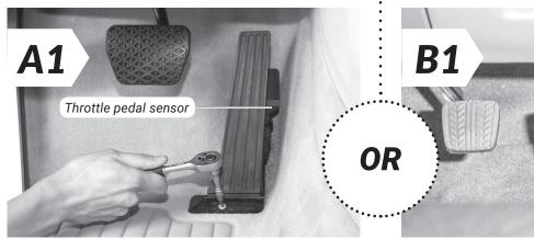
• Disassemble the throttle pedal with the appropriate tools.
