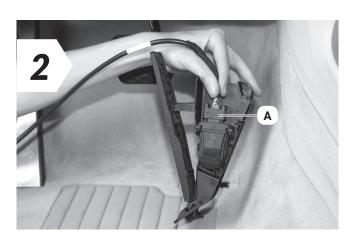
Attach connector A from the Brainbox to the gas pedal sensor.
