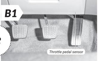
Disassemble the throttle pedal with the appropriate tools.
