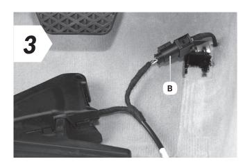
Now attach connector **B** to the connector you pulled off the gas pedal.
