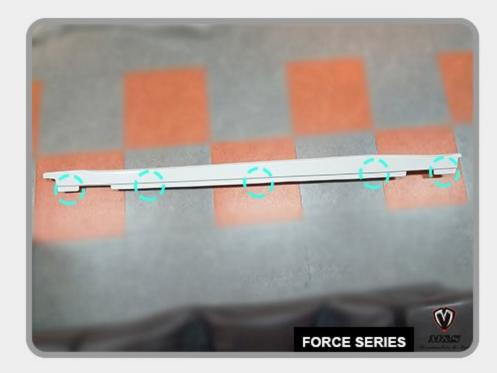
Fix the side lip with screws from bottom of the vehicle on the positions circled in blue.
