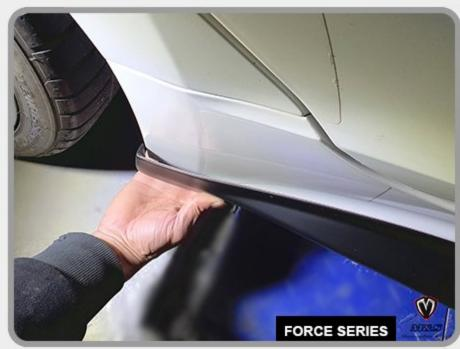
4. Remove the protective film on the double-sided tape and fit the side lip as shown.
