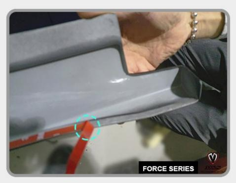
2. Peel just enough of the protective film on the double-sided tape so you can hold on to the film by hand.
