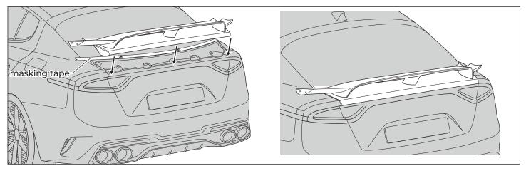
C-4. Remove the masking tape and secure the [end plates] in the correct position using the provided [hex bolts]. Note, that excessive torque can cause deformation and damage.
