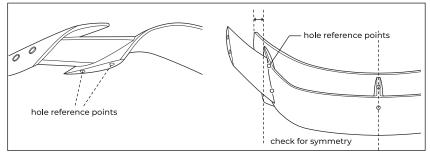
A-3. Mark the position with masking tape.
