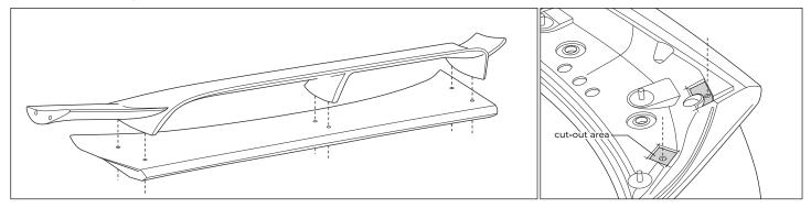
C-2. Secure the spoiler to the trunk cover using the provided [bolts] and [washers] with appropriate torque.
