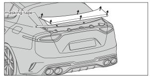
A-2. Position the carbon fiber rear spoiler over the trunk cover and check the alignment.
