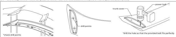
B-2. Using either a grinder or a hole saw, cut through the bottom of the trunk cover in the areas shown below to create space for the hex bolts (total 6 places).
