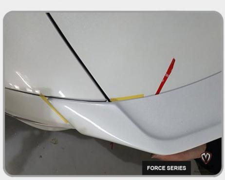
Place the spoiler on the trunk and position it to the installation location marked in step 1.
