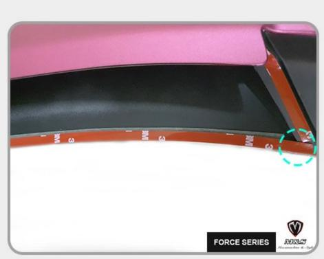
4. Remove the protective film of the tip of the 3M double sided tape shown in step 3, then add additional 3M double sided tape all the way to the end of the spoiler as shown in the above photo.
