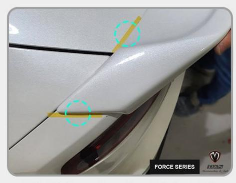
Test fit the spoiler and mark the installation location with masking tape as shown in the above photo.
