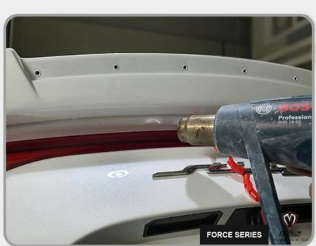
8. If the spoiler is being installed at a low temperature area, applying low heat using a heatgun will enhance the adhesiveness of the 3M double sided tape.
