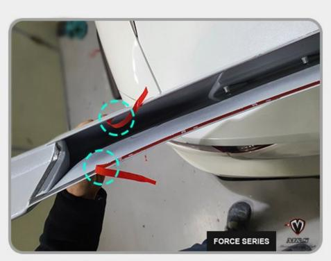
Peel off a bit of the protective film of the 3M double sided tape as shown in the above photo, so that it can be pulled off fully once the spoiler is in the correct position for installation.
