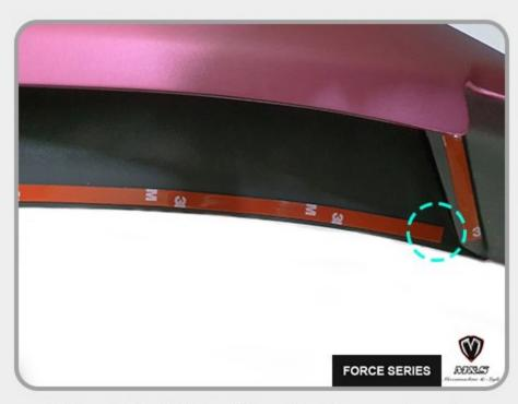
Apply the 3M double sided tape up to where indicated in the above photo.
