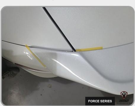
7. Remove the protective film of the 3M double sided tape fully, and firmly press the spoiler to complete the installation.
