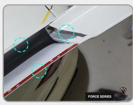
Apply the 3M double sided tape on the inside of the spoiler as shown in the above photo.
