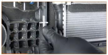
**68.** Transfer the top grommets from the stock intercooler to the Mishimoto intercooler.
