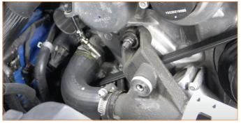
37. Remove the nuts that secure the blow-off valve pipe. (2x 14mm nuts)
