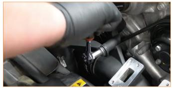
58. Tighten all the clamps on the pipe.
