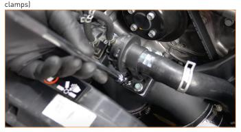
60. Reconnect the vacuum line to the cold-side pipe. (1x spring clamp)
