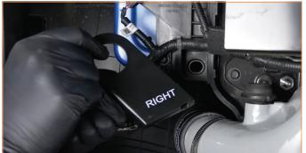
**75.** Bend the ambient temperature sensor bracket back to its original position.
