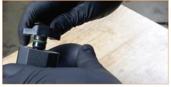
55. Install a coupler to the throttle body. (1x worm gear clamp)
