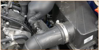
**33.** Separate the second vacuum line attached to the intake from the engine port. (1x spring clamp)
