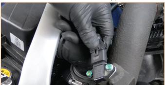
**27.** Loosen the clamp where the cold-side coupler meets the throttle body. (1x tamper-proof cap, 1x worm gear clamp)
