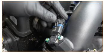
**63.** Install a coupler to the cold-side intercooler pipe. (1x worm gear clamp)
