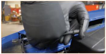
**04.** Remove the clips that secure each wheel well liner and the bolts on the upper edge of the bumper. (6x pop-clips, 2x 10mm bolts)
