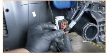
18. Disconnect the electrical harness for the smart cruise control radar
