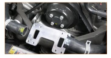
**25.** Remove the bolt that secures the bracket for the cold-side pipe. (1x 10mm bolt)
