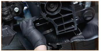
51. Tighten the clamp at the bottom of the blow-off valve pipe.
