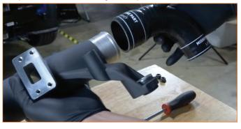
**46.** Install the couplers on the Mishimoto blow-off valve pipe to the turbo outlets and align the grommets on the pipe to the studs on the front of the engine. (2x 14mm nuts, 2x worm gear clamps)
