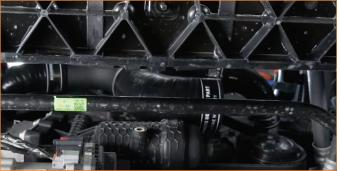
49. Slide the hot-side pipe into the coupler installed in the previous step.
