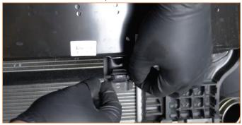
**16.** Disconnect the electrical harnesses for both horns and the hood latch.
