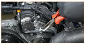
**34.** Loosen the hose clamp on the driver-side intake tube. (1x worm gear clamp)
