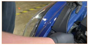
03. Remove the bolts that secure the top corners of the bumper. (2x
