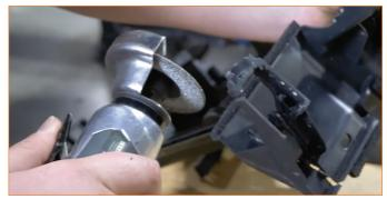
43. Cut across the lines drawn on the sides of the ducting.
