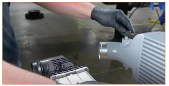
69. Place the bottom grommets in the brackets on the vehicle.
