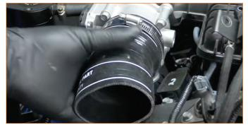
**56.** Feed the cold-side intercooler pipe down toward the intercooler.
