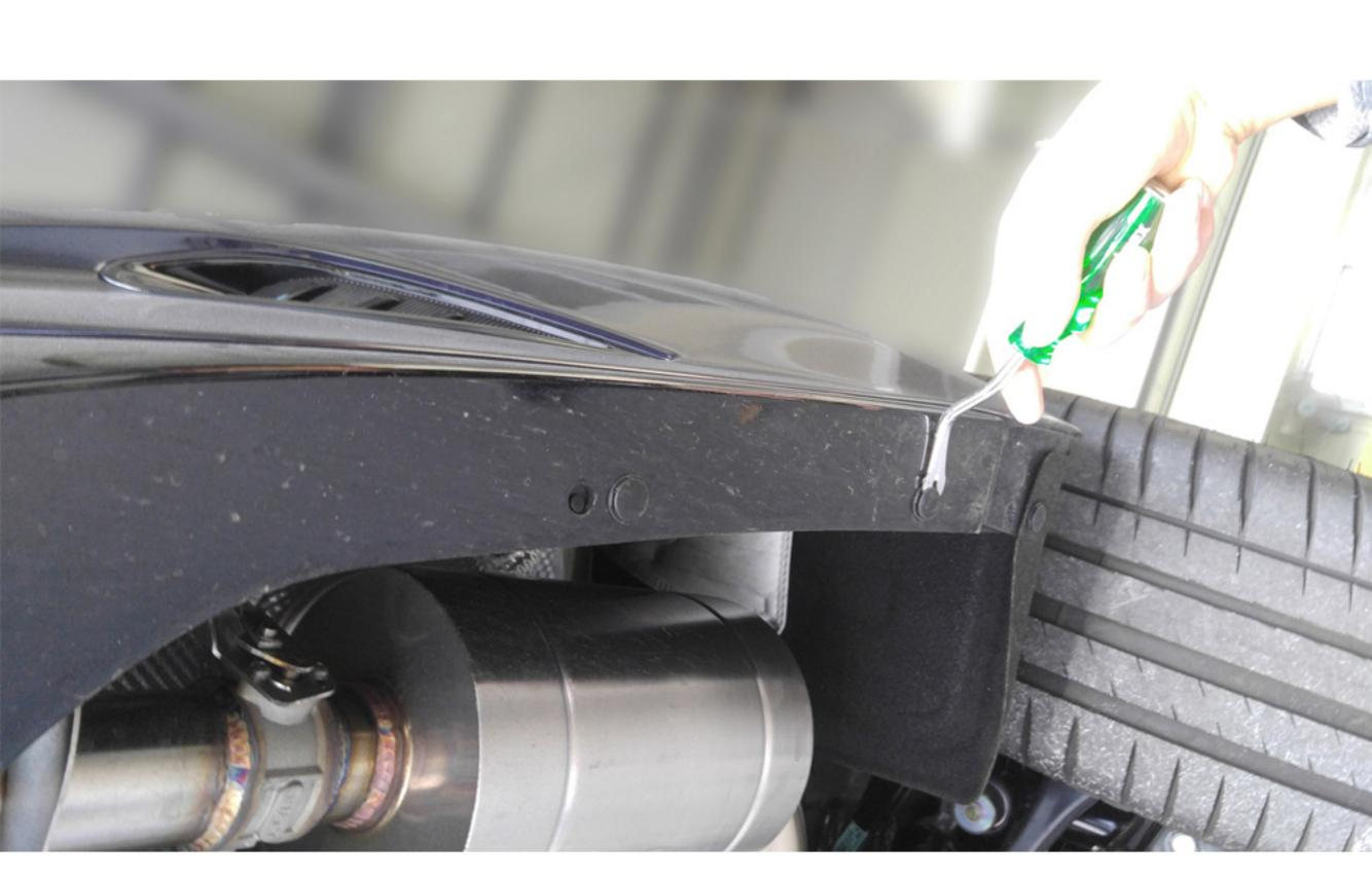
1. Remove 3 factory pins from the bottom panel
