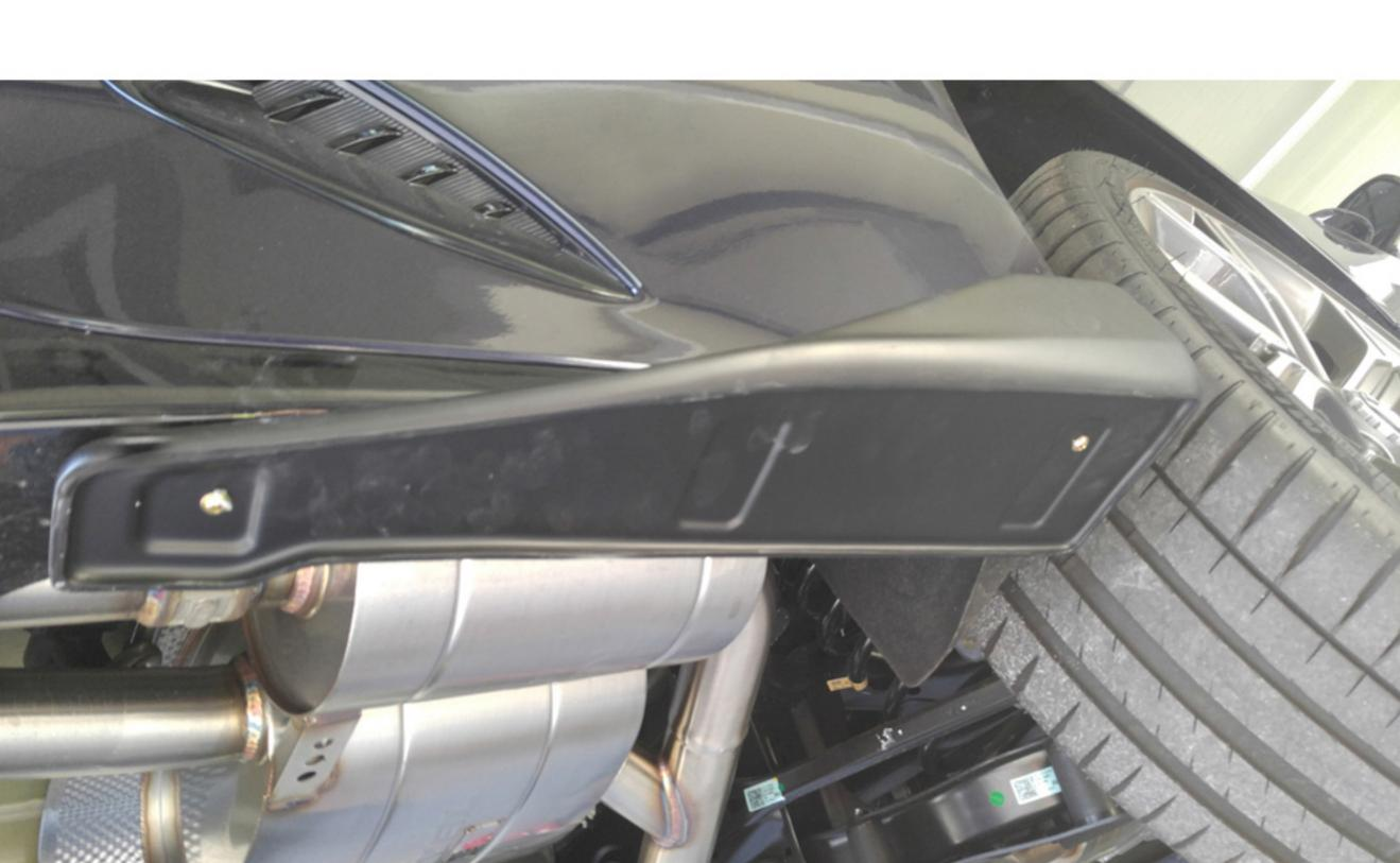
2. Test fit the rear lip pieace to the desired location and mark all spots for drilling
