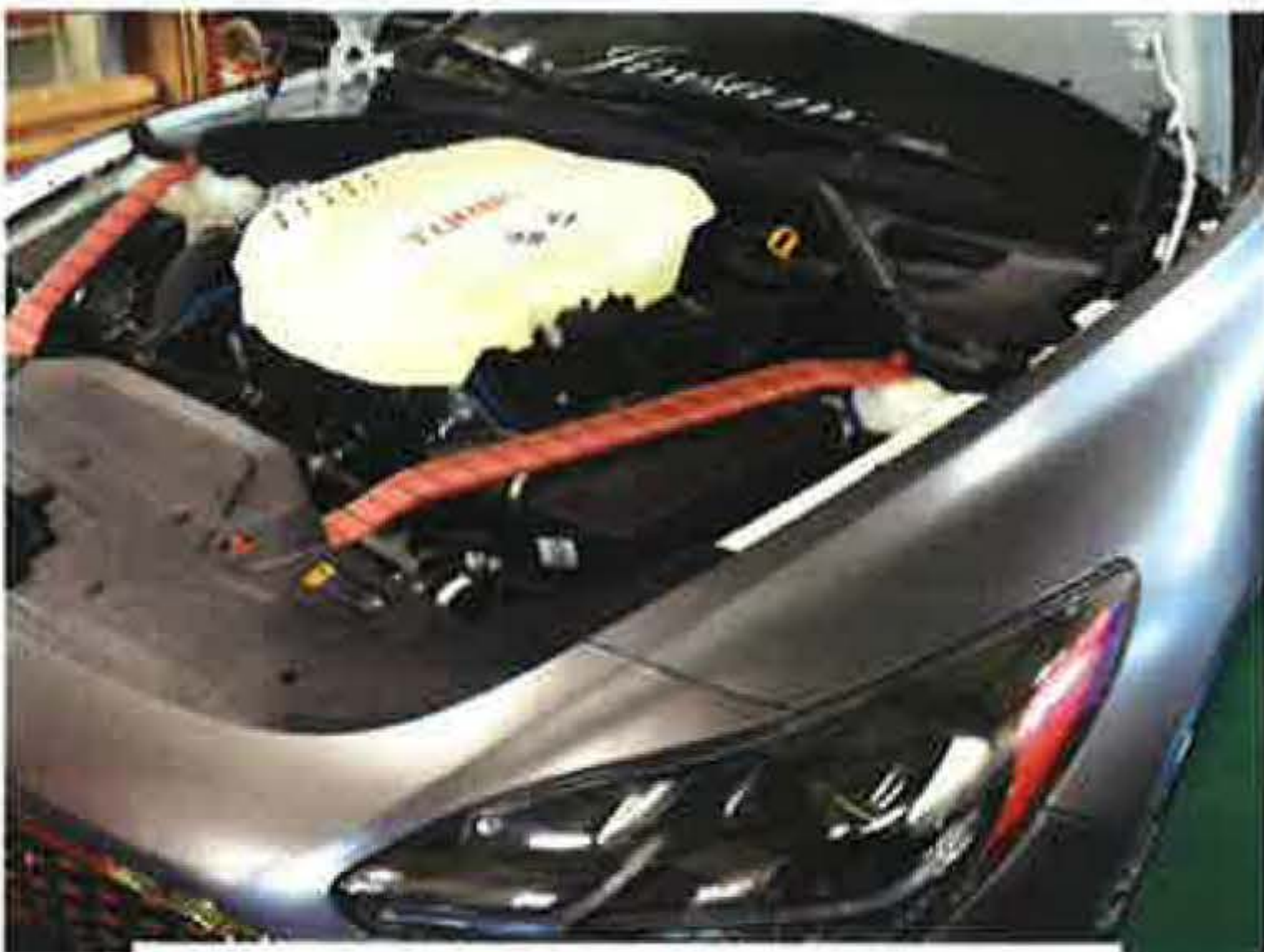
Loosen the bolts on the marked bar and remove the all bars
