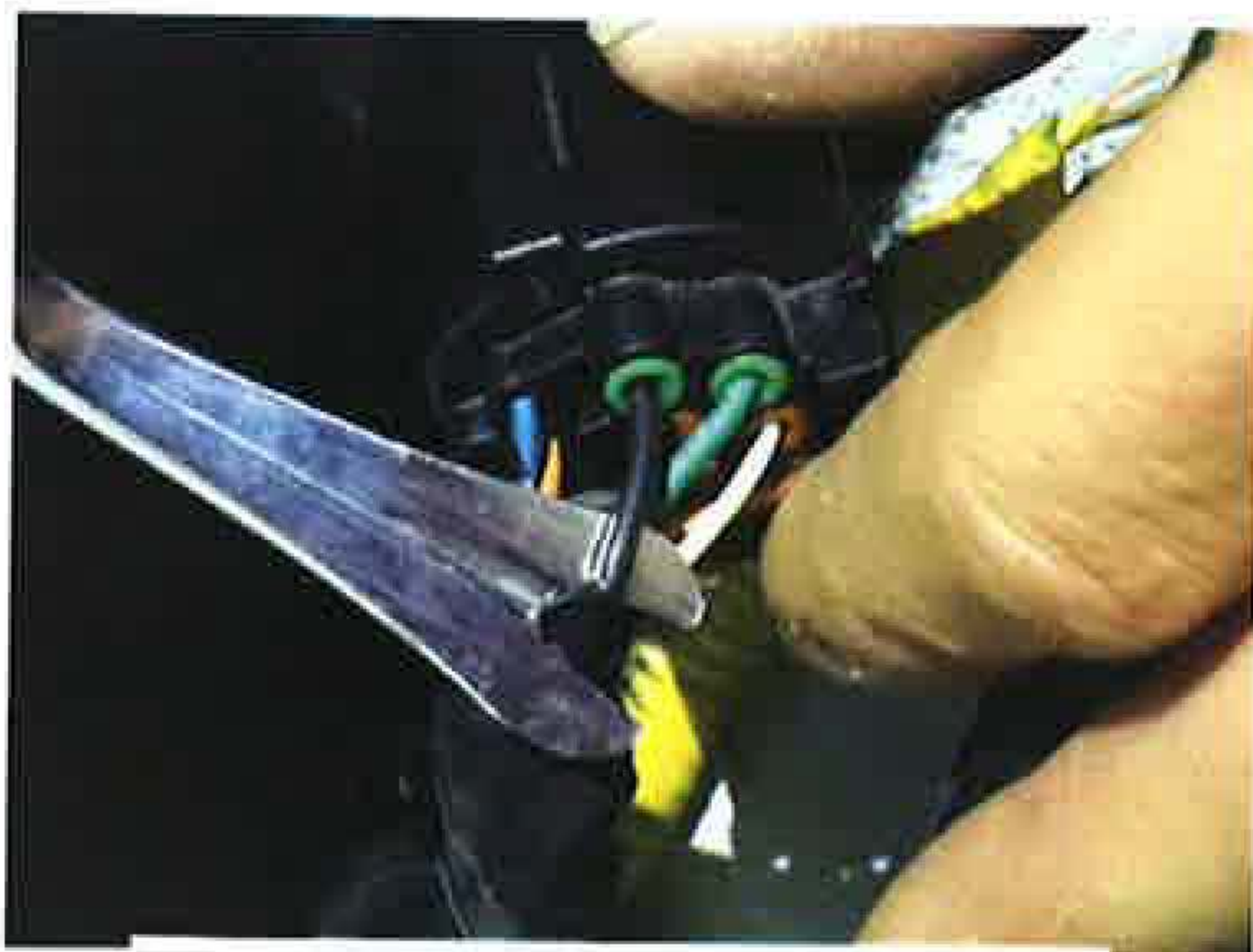
Connect the goods Black wire(-) to the car's Black wire
