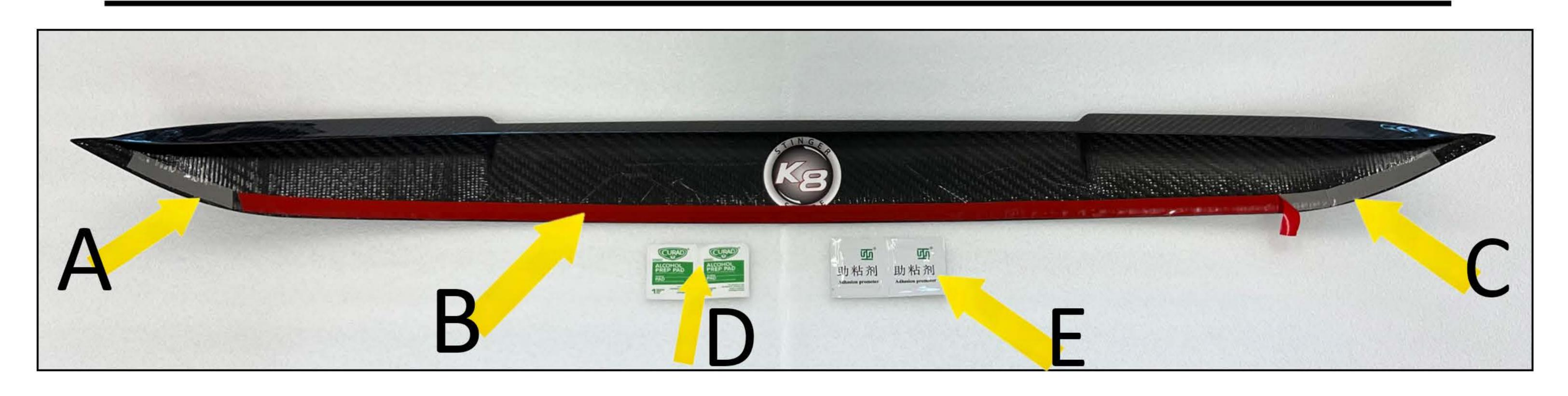
STEP 1: CLEAN WINDOW AND WIPE DOWN AREA WITH AN ALCOHOL WIPE (D)
