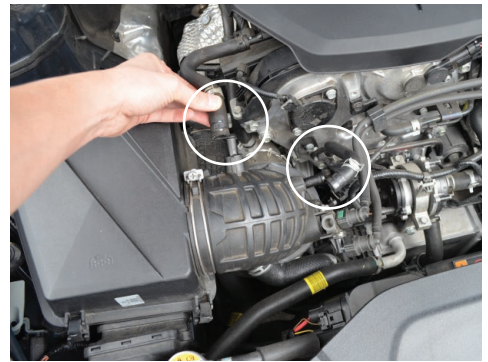
3. Disengage the tensions clamps securing both crank case hoses on top of the tube, then detach both crank case hoses.
