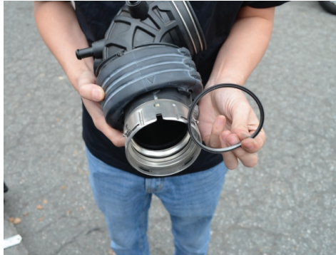
17. Remove the O-Ring from the intake tube. Take note of the direction it is removed in.
