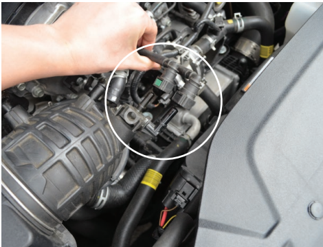
4. Detach both evap lines by holding the release button, then pulling the lines away from the evap fitting.
