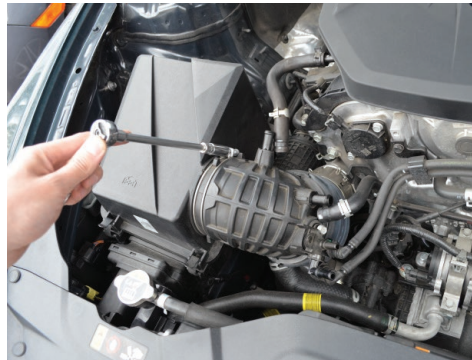
5. Loosen the clamp securing the intake tube to the airbox.
