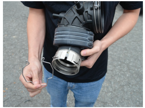
15. Remove the C-Clip from the oem intake tube.
