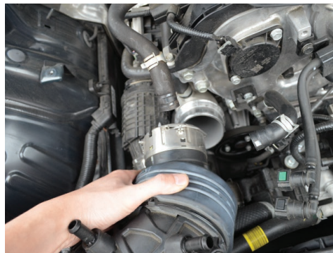
8. Disengage the C-Clip securing the intake tube to the turbo, then detach the intake tube.
