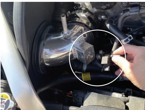
22. Install the evap fitting onto the intake tube. Ensure the O-Ring is still on the evap fitting.
