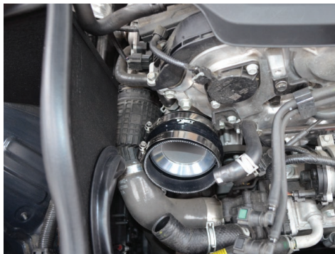
20. Attach the 4.00" hump hose onto the turbo inlet adapter. Secure the hose with the provided clamp.
