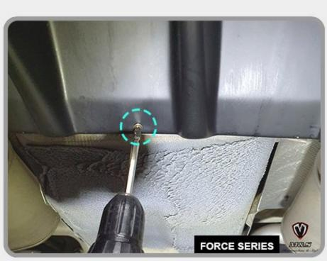
7. Fix the underneath of the center piece of the Rear Diffuser with screws as shown.
