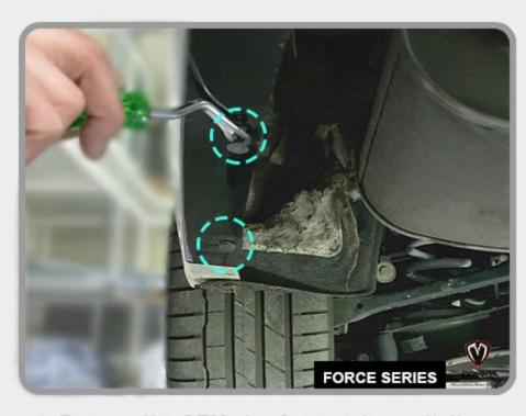
1. Remove the OEM pins from underneath the vehicle as shown.
