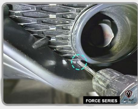
6. Fix the bottom of the center piece of the Rear Diffuser with screws as shown.
