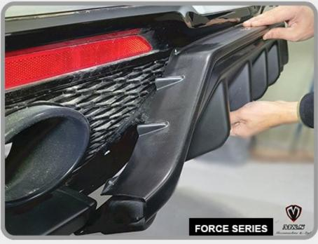
5. Align the center piece of the Rear Diffuser from top to bottom as shown.
