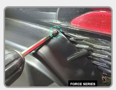
6. Fix the top of the center piece of the Rear Diffuser with screws as shown.
