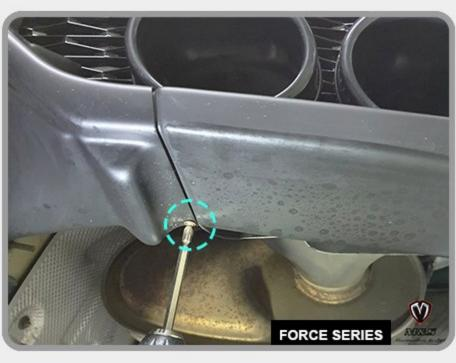
8. Fix the position where the both side pieces and the center piece of the Rear Diffuser connect with screws as shown.
