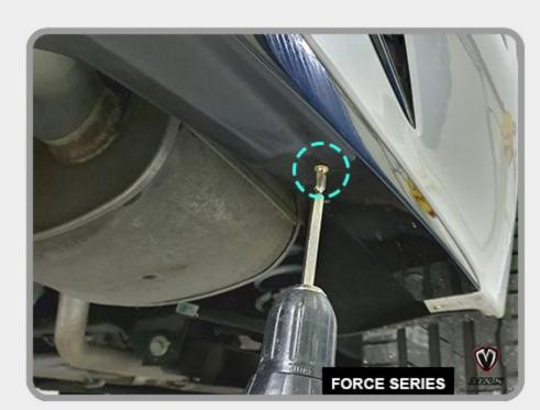
4. Fix the rear part of the pieces with screws as shown.
