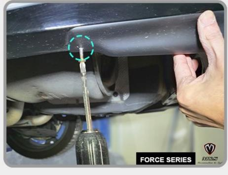
3. Fix the front part of the pieces with screws as shown.
