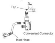
The convenient connector may not fit all faucets. You may need to twist the tip off or add an adapter to fit properly.
