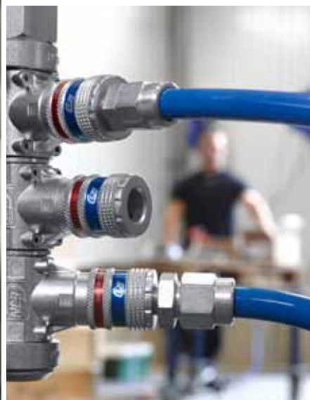
eSafe vents the down streaming pressure before disconnection reducing noise level and the risk of operator injury during tool change.
