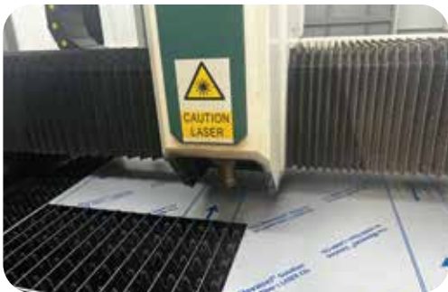
Fibre Lazer steel machine cuts tags and plates from steel sheeting.
