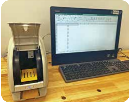
Smartmark printer "plug and play" uses excel to input then export data for printing.
