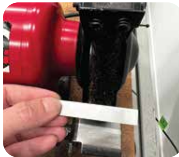
Steel tags & plates are then buffed/polished and deburred.
