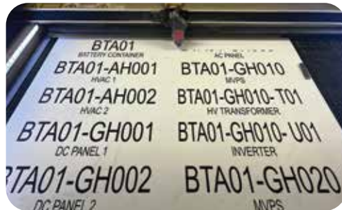
CO2 Lazer printing on Smartlaze industrial Traffolyte sheet.
