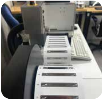
Fibre lazer printer, etches images onto SS cable tags effortlessly.
