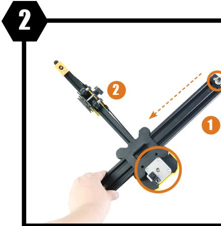
Slide the profile of the **Y axis** through the guiding wheels of the **X axis**.
