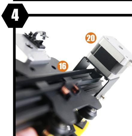
Pass the **belt** through the synchronization wheel of the **Y axis** and the **motor** installed in the previous step.
