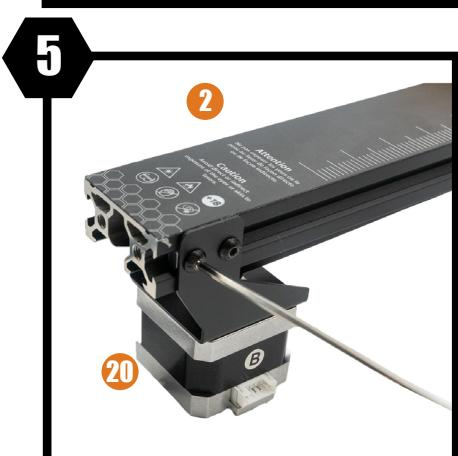
Position the **motor block** as close as possible to the edge of the **Y axis**.
