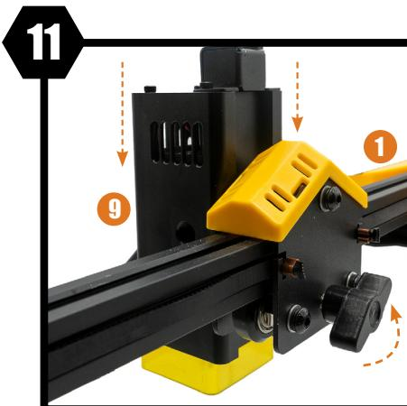
Loosen the screw at the back of the platform on the **X axis**.
