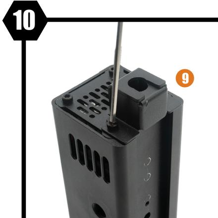
Unscrew the **2 screws** above the **laser head**.
