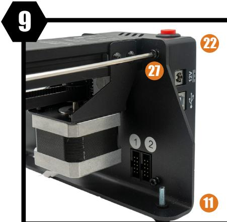
Use the **4 screws** and **washers** to secure the **enclosure** to the **foot**.
