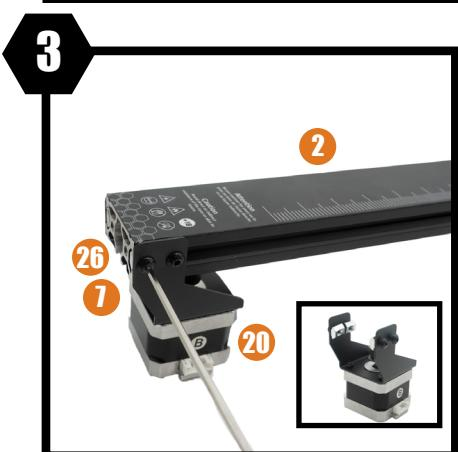
Prepare the **4 screws** by inserting them through the **motor bracket** and add **one nut** to each screw. Insert the nuts into the profiles of the **Y axis**.
