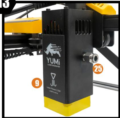
Screw the **nozzle** into the **laser head**.
