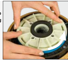
Figure 6 Unscrew the top stone by turning it counterclockwise.
