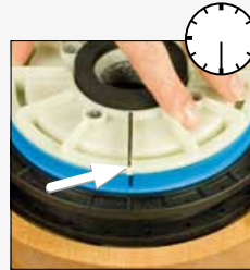
Figure 7 The black marks must be located over one another.
