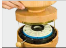
Figure 2 Lift off the funnel.
