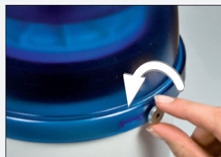
Figure 3 Turn the funnel slightly to the left with both hands (counterclockwise) and lift it up.
