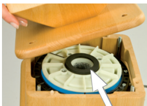
Figure 4 Make sure the foam rubber gasket is properly seated (arrow). Now return the funnel to its previous position and secure it with the brass screws
