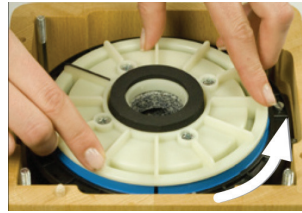
Figure 6 Remove the top grindstone by turning it counter-clockwise
