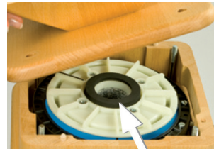
Figure 9 Make sure the foam rubber gasket is properly seated (arrow). Return the funnel to its previous position and secure it with the brass screws
