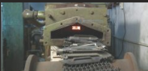
Controlled atmosphere hardening & tempering line to achieve optimal hardness for Blades & Peelers, ensuring longer lasting edge.
