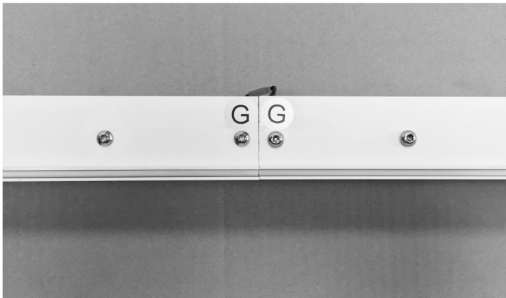
Connect G, again connecting the power jumper as previously.
