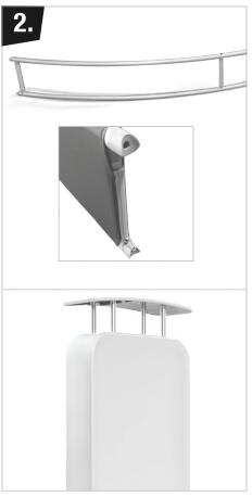
Keeping the towers and rings separate, slide on each of their graphic prints like a pillow-case. Attach the monitor mounts as shown using the 4 screws provided. After that, zipper at the tower bottoms and ring sides.
