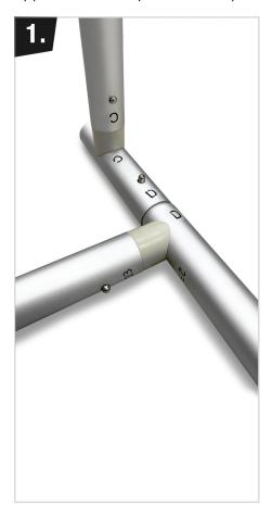
Separately assemble the frames for the towers and the partial rings. Connect the poles and match the symbols together. Click together so the button nubs protrude through the holes.
