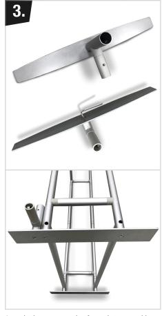
Attach the pegs to the feet plates used by the back wall and arch using the provided bolts. Use the hand tool included to tighten it. One tower foot that has 3 pegs/extensions on it — two of these pegs are used by the tower, and one is used by the left side of the back wall. Attach the feet to the frames.
