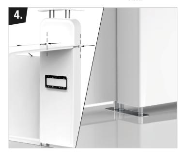
Find the small hidden zippers in the seams shown by the arrows. Carefully open these so that you can get hands into the tower. Bolt the arch to the tower, from the tower interior, through the tower horizontal pole, through the premade button holes in the fabric, into the arch pole ends. Place the right side of the back wall on the 3-peg shared foot with the tower.
