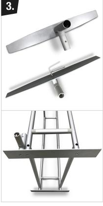
Attach the pegs to the feet plates used by the back wall and arch using the provided bolts. Use the hand tool included to tighten it. One tower foot that has 3 pegs/extensions on it — two of these pegs are used by the tower, and one is used by the left side of the back wall. Attach the feet to the frames.
