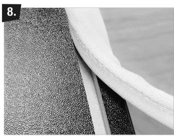
Insert the silicone graphic edge into the groove, going all around the table top. Then turn the table upside down, and do the same for the bottom-side silicone edge.
