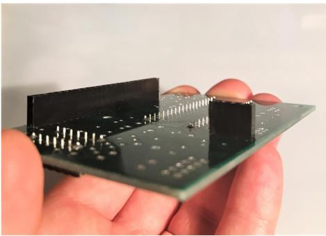
Once seated correctly, solder the remaining header strip pins.
