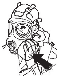
NEGATIVE PRESSURE LEAK TEST
