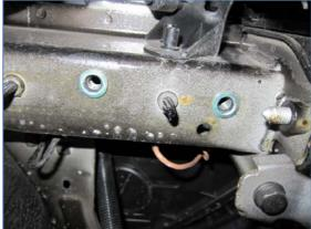
5. Reload the rivnut tool with the unused greased bolts and rivnuts. For the passenger side you will use the hole on the end with a single hole PLUS the unused hole on the other end. Repeat the setting process on the passenger side. A 12" wobble extension or universal joint on the socket is very helpful to drive the bolt heads since access directly below the bolts restricted. Remove the bolts and tool once the rivnuts are set.
