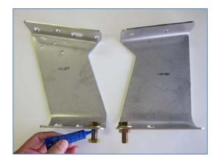
5. Shake the provided tube of threadlocker vigorously. Unscrew the white cap and cut the tip off of the tube of threadlocker at the embossed ridge near the tip of the tube. Place one drop of thread locking compound on each of the 12mm x 30mm bolts at about the point where the nut will sit on the other side of the mounting bracket (see picture above).
