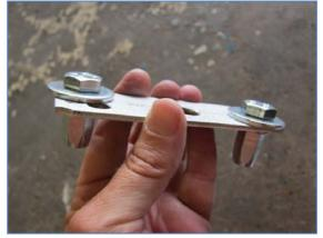
3. On the driver side of the car, push the hex rivnuts into the two hex holes in the underside of the frame rail. The rivnuts will likely need to turn a little to line up with the hex holes in the frame rail.
