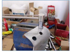
The protruding section of the two 12mm bolts will be the forward mounting points of the Dieselgeek Panzer Plate:
