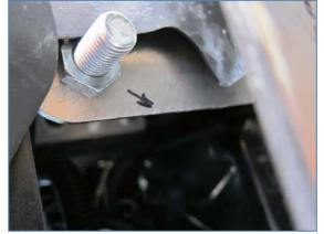
4. Once the plate mounts are correctly adjusted, you will need to notch the side plastic pieces to allow the 12mm jam nuts to be fully exposed so that the skid plate can be mounted to the studs with no plastic in the way.
