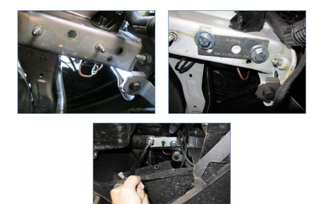
4. Once the tool and rivnuts are flush with the frame rail, partially tighten one of the bolts with your 17mm socket, 12 inch extension and ratchet. Push up on the socket slightly as you tighten the bolts so that the rivnuts remain flush with the frame rail. Repeat for the other bolt but tighten slowly until it gets noticeably harder to turn. Repeat for the other bolt. Once both rivnuts are set, remove the bolts and rivnut tool from the frame rail.
