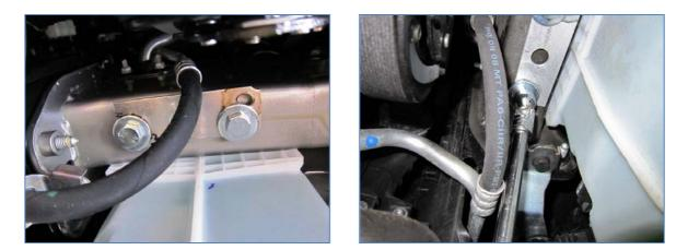
6. Attach the left and right mounting brackets to the installed rivnuts by using the greased 10mm bolts. Leave the bolts ever so slightly loose so that the mounting brackets can be moved during the trial fitting of the skid plate. Please note that the threaded 8mm stud or studs on the driver side will not be used to attach the mounting bracket.
