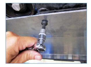
3. Try to engage the two front studs with the two front holes in the skid plate. If the plate goes on easily then you will not need to adjust the position of the front mounting brackets.
