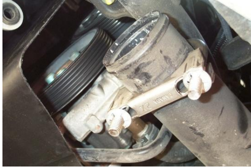
Figure 22 – Retainer Disc on the Threaded Stud
