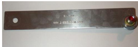
Figure 33 – Greased Bolt in Offset Hole
