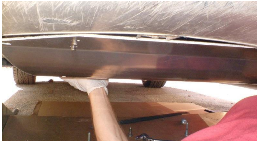
Figure 34 – Line Up the 1/2 Inch Skid Plate Holes
