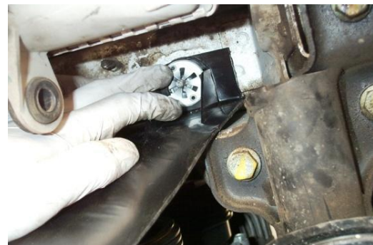
Figure 19 - Star Washers of the New Side Panel on the Threaded Stud Mounts
