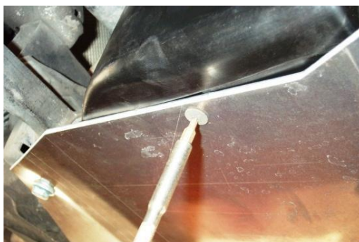
Figure 36 - Attach the Vertical Engine Bay Side Panels
