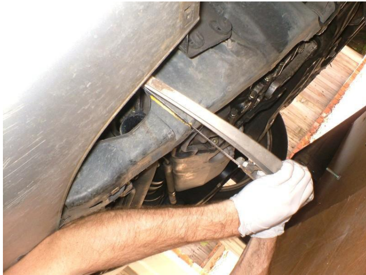
Figure 11 – Removing Forward Section of Side Panel
