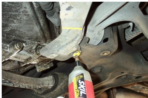
Figure 9 - Removing the Rear T25 Torx Screw
