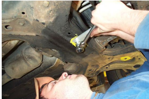
Figure 35 – Rear Center Hole of the Subframe
