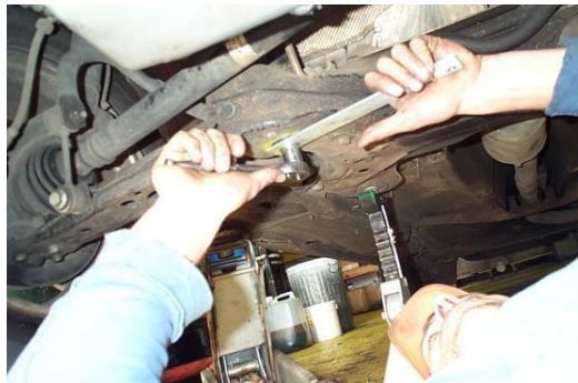
Figure 34 - Tightening the 10mm Bolt
