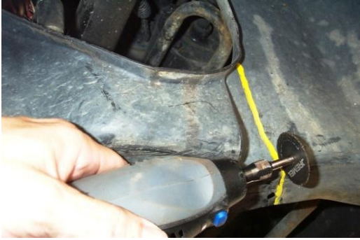
Figure 12 – Using Dremel Tool to Cut Side Panel
