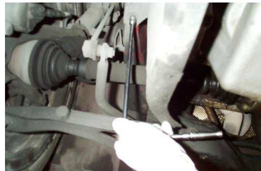
Figure 15 – Removing the Sheetmetal Nut
