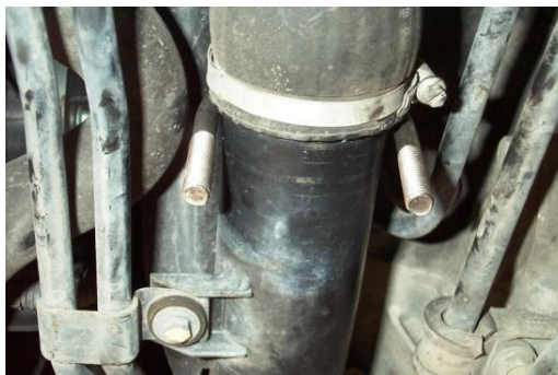
Figure 21 - Exhaust Clamp U-Bolt over the Steel Intercooler Tube
