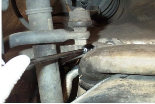
Figure 16 - Access the Rear 10mm Nut
