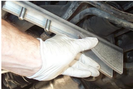
Figure 25 - Engage the U-Bolt Studs with the Aluminum Mounting Bracket
