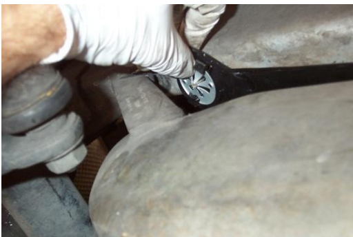
Figure 18 – Installing Star Washers
