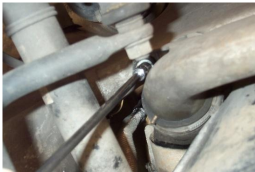
Figure 17 - Removing the Rear 10mm Nut
