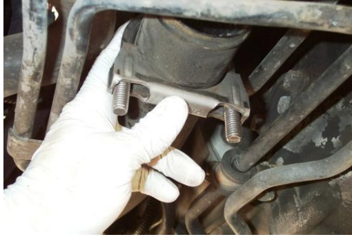
Figure 24 – Sheet metal Part Of The Exhaust Mount Up Against The Intercooler Tube.
