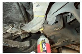
Figure 9 - Removing the Rear T25 Torx Screw
