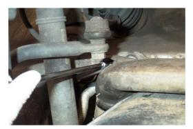
Figure 16 - Access the Rear 10mm Nut
