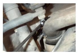
Figure 17 - Removing the Rear 10mm Nut
