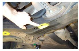
Figure 31 - Center 13mm Hole Pre-Drilled In the Subframe
