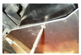
Figure 36 - Attach the Vertical Engine Bay Side Panels
