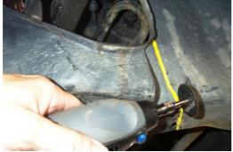
Figure 12 – Using Dremel Tool to Cut Side Panel
