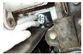
Figure 19 - Star Washers of the New Side Panel on the Threaded Stud Mounts
