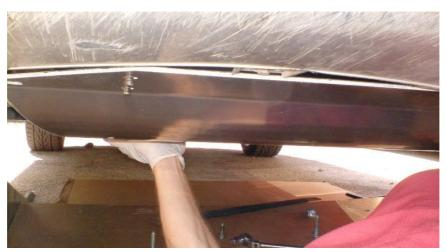
Figure 34 - Line Up the 1/2 Inch Skid Plate Holes
