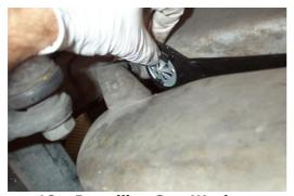
Figure 18 – Installing Star Washers
