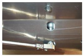
Figure 35 - Two Oblong Holes in the Skid Plate
