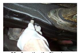
Figure 30 – Inserting the Rivnut
