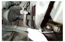
Figure 15 – Removing the Sheetmetal Nut
