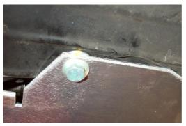
Figure 29 - Large Washer Used As a Spacer
