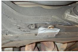
Figure 33 - Use a Small Piece of Duct Tape to Fix Rivnut in Place
